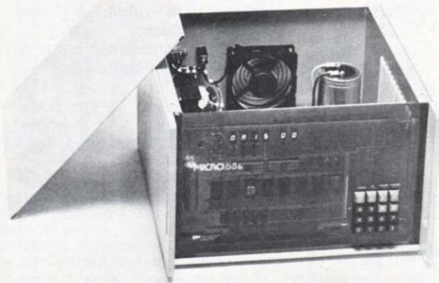
Photo 3. The Electronic Product Associates Micro-68b, a larger version of the original Micro-68. A printer, TV interface, cassette interface and floppy-disk system are available with this computer. (Courtesy of Electronic Product Associates)
